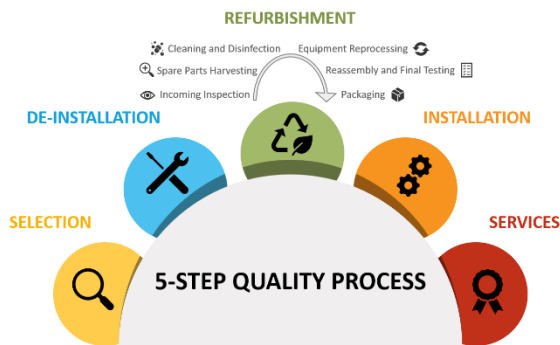
Figure 1. 5-Step Quality process to refurbish a medical system according to the case-study company, and in accordance with the NEMA/MITA standard for refurbishment.
